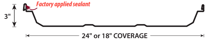
Central-Loc® - 3" Snap-lock Recommended minimum pitch - 1/4:12 | Purlin spacing - 5'
